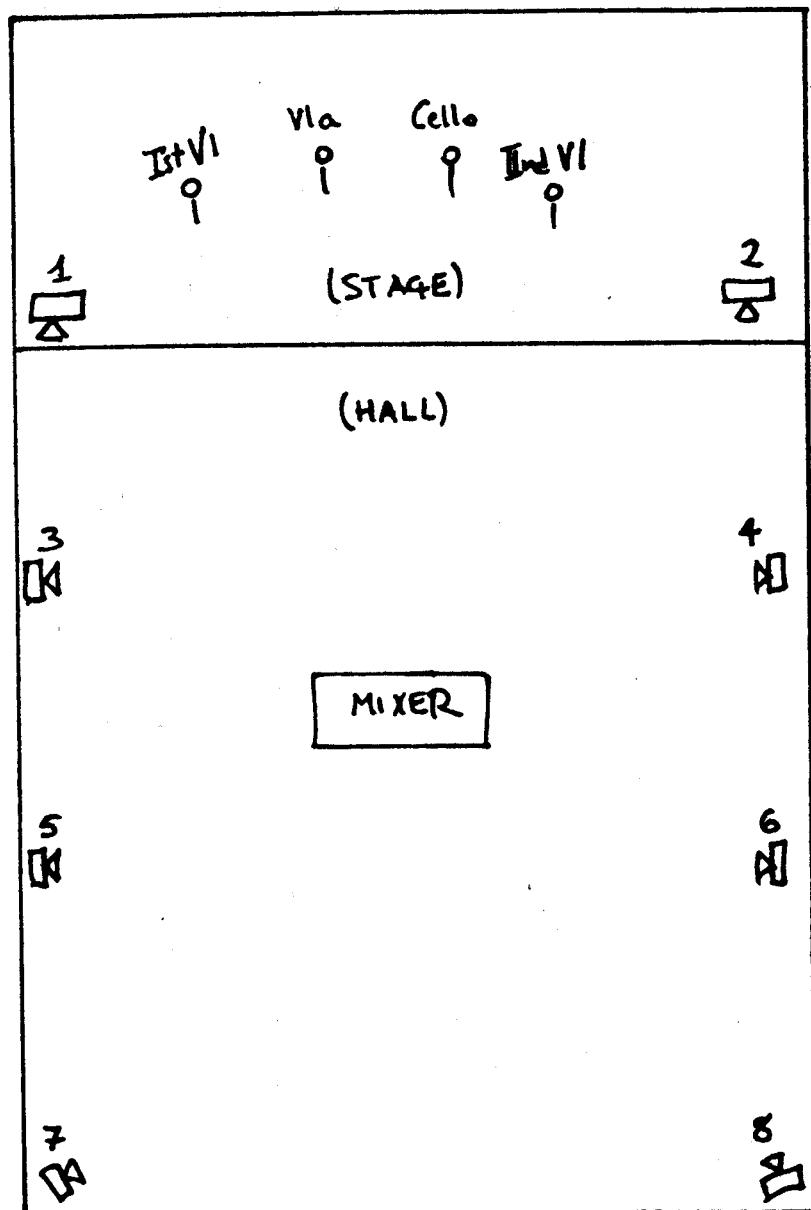
STRING QUARTET: Placed along a loose arch, the instruments should be distant enough so as to assure a good pick up with little diaphony.
